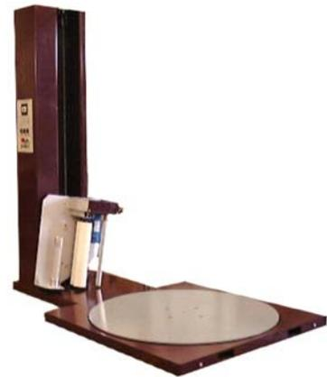
**High Profile Turntable** - The high profile machine has a raised turntable, usually 11" - 12" from the floor to the turntable, and can only be loaded with a forklift truck! There is no possibility of loading a high profile machine with a pallet jack. The high profile machine can be interfaced with a pallet conveyor line to feed pallets directly onto the wrapping machine turntable.
